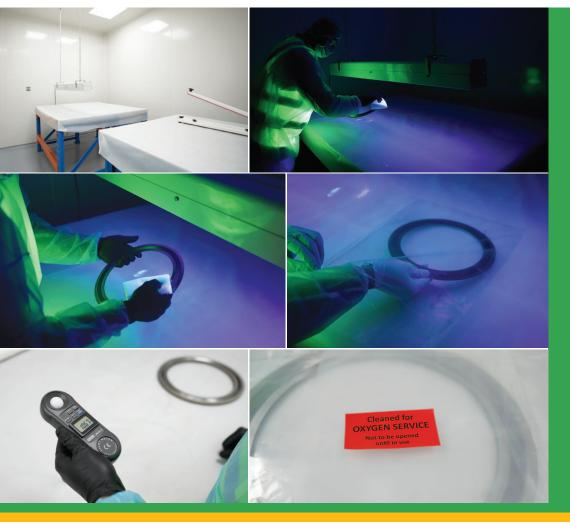
Flexitallic has invested in its Ras Al Khaimah, UAE manufacturing facility to support Middle East and Africa customers by installing a ISO Class-7 validated clean room to supply Oxygen Cleaned Gaskets in line with the CGA G-4.1 procedure.
